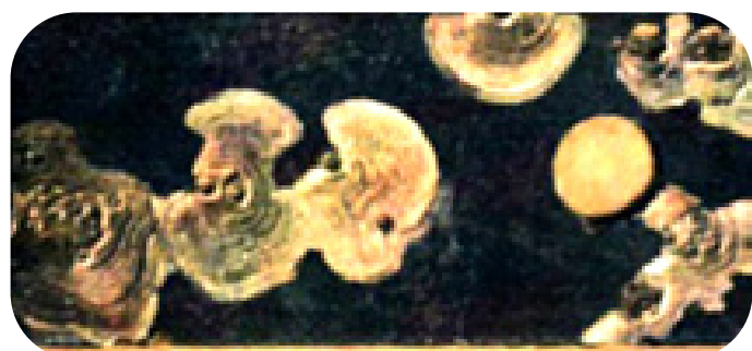
Figure 1: The left photo shows a cleaned low-carbon steel corrosion coupon with SRB growing on it and producing concentric rings of corrosion. The right photo is a water washed Type 304 stainless steel 5/8 inch condenser tube that has pits and dark spots. 4 Source: Understanding and Detecting MIC in Cooling Water Systems ; Paul R. Puckorius 5
