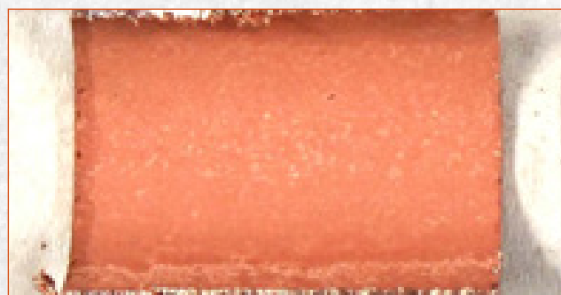
Fig 3 – Same Specimen after 6 hours immersion with stirring in 2% ammoniated citric acid solution
