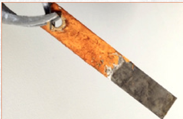
Fig 1 – Mild Steel Test Coupon following 12 hours part immersion in a stirred chelant based cleaning agent at 3% concentration
