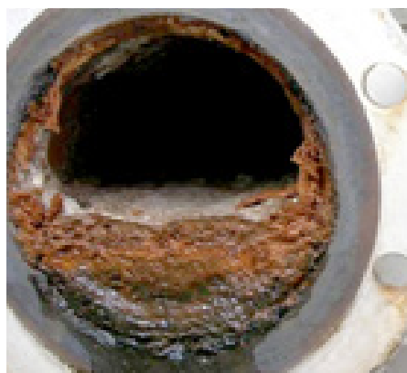
Scale, biofilm, and corrosion deposits within pipework
