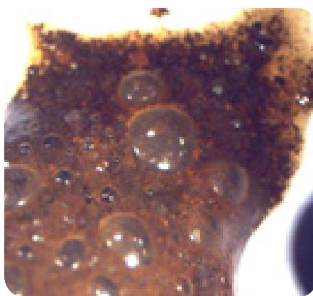
Figure 7: High rate of Nitrogen bubble evolution showing, indicating positive indication of SRB Source: Microbiologically Induced Corrosion ; Ibraheem, Ameer K 8
