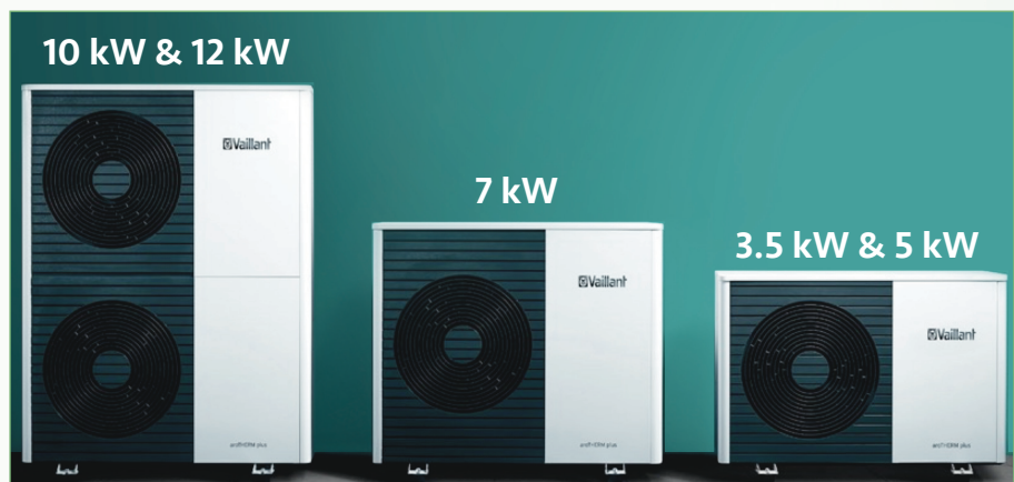
Figure 7: Heat Exchanger size versus heat pump power. If we wish to harvest heat from air at a greater rate, it is necessary to have physically larger heat exchangers. The graphic shows a range of heat pumps from Vaillant and their maximum rates of heat delivery. Heat pumps of all manufacturers are of a similar size.
